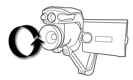
Aim the IR camera at the subject, turn the focus ring to focus on the target.
