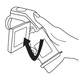
Open the LCD displayer in the direction of the arrow.
